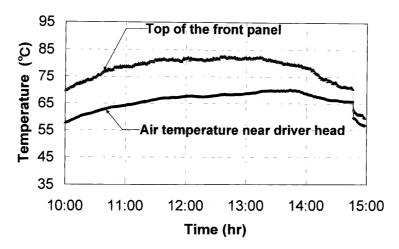
Fig. 3 Temperature variation with time at different locations (without cooling)
