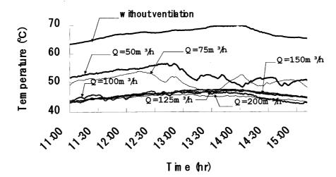
Fig. 4 Temperature variation with time at different flow rates (m<sup>3</sup>/h)
