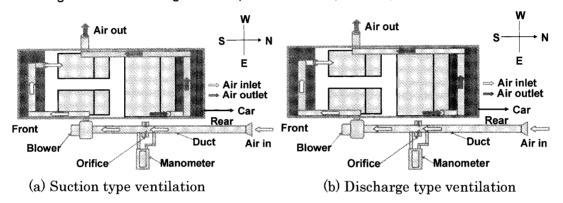
Fig. 2 Schematic diagram of experimental setup for flow rate measurement
