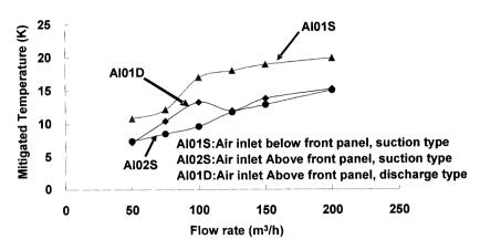
Fig.5 Effect of different air inlet locations and different ventilation methods on temperature mitigation
