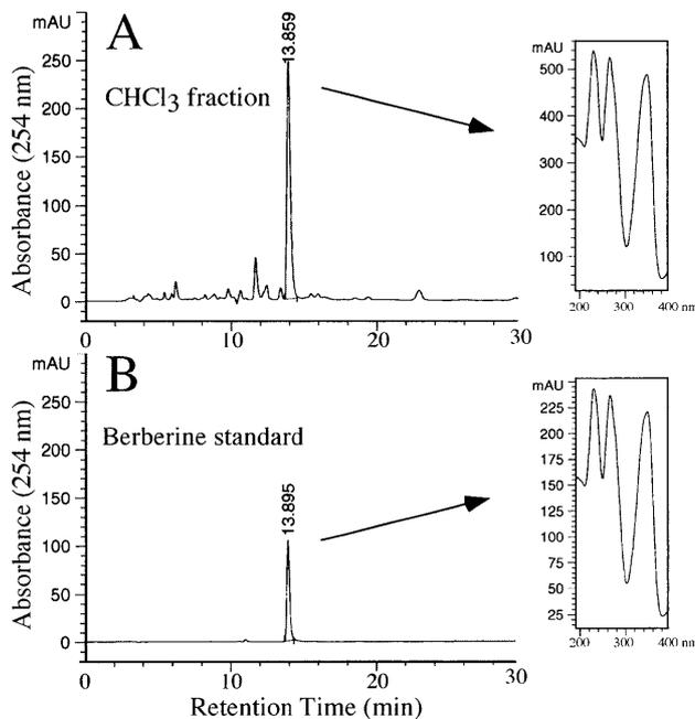
**Fig. 5.** High-performance liquid chromatography (HPLC) patterns of CHCl<sub>3</sub> fraction from decocted extract of Coptidis Rhizoma and standard sample of berberine. Data are expressed as mean ± s.d. (n=4).
