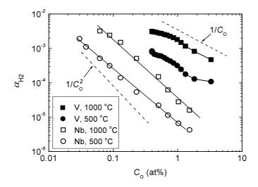
Fig. 4 Comparison of  $\alpha_{H2}$  between V and Nb [7].
