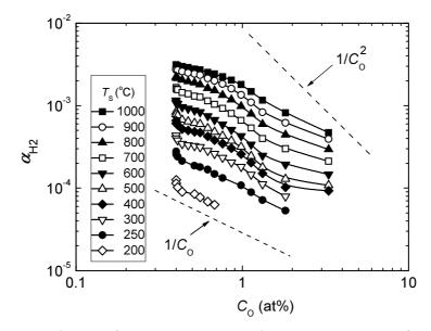
Fig. 3 Dependence of  $\alpha_{H2}$  on  $C_O$  at various  $T_S$ . Pressure of H<sub>2</sub> gas in upstream side was 0.4 Pa.
