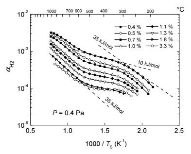
Fig. 1 Temperature dependence of sticking probability  $\alpha_{H2}$  on V surface at different oxygen bulk concentration  $C_O$  indicated in the figure. Pressure of H<sub>2</sub> gas in upstream side was 0.4 Pa.
