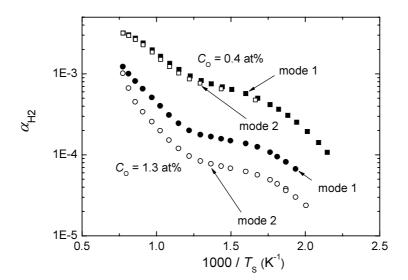
Fig. 2 Influence of thermal history of specimen on  $\alpha_{H2}$ . Solid symbols refer to  $\alpha_{H2}$  measured by keeping specimen at given temperatures for 10 min (mode 1), whereas open symbols refer to  $\alpha_{H2}$  obtained by holding specimen for sufficiently long time (mode 2). Pressure of H<sub>2</sub> gas in upstream side was 0.4 Pa.
