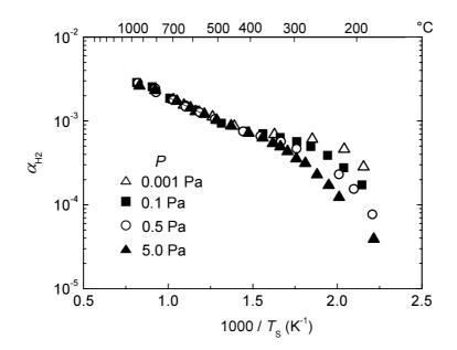
Fig. 5 Temperature dependence of  $\alpha_{H2}$  on V surface at various H<sub>2</sub> pressures  $(C_{O} = 0.4 \text{ at.}\%)$ .
