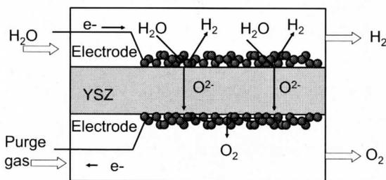
Fig.1 Schematic diagram of principle of ceramic electrolysis method
