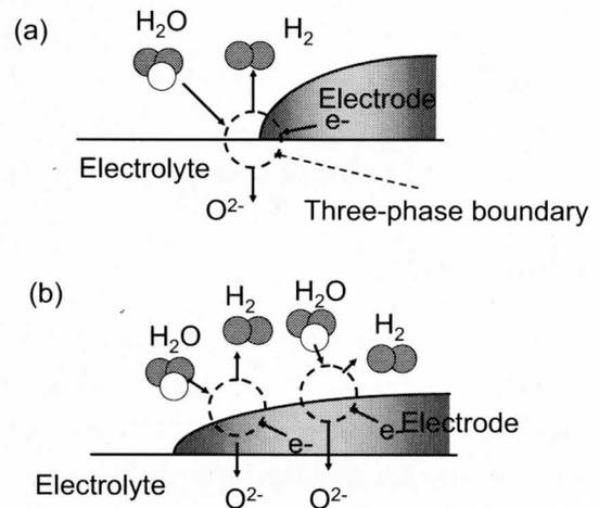
Fig.2 Schematic diagram of reaction point
