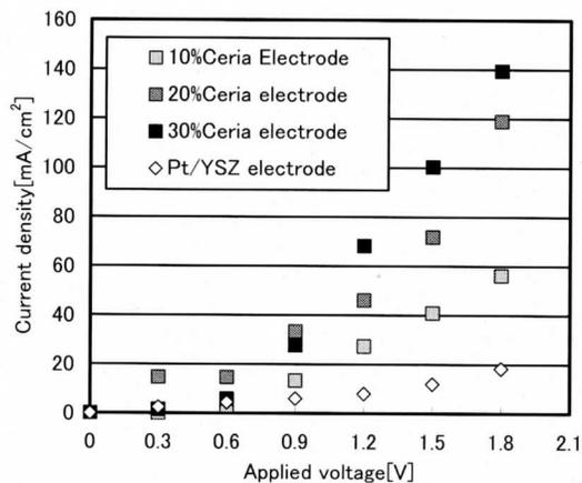
Fig.3 Current density of electrodes against applied voltage
