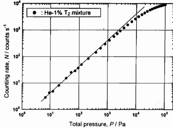
Fig. 4 Pressure dependence of X-ray intensity for the He-1%T<sub>2</sub> mixture.
