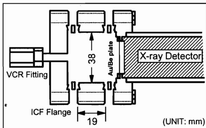
Fig. 1 Cross-sectional view of the measuring cell for gaseous tritium.
