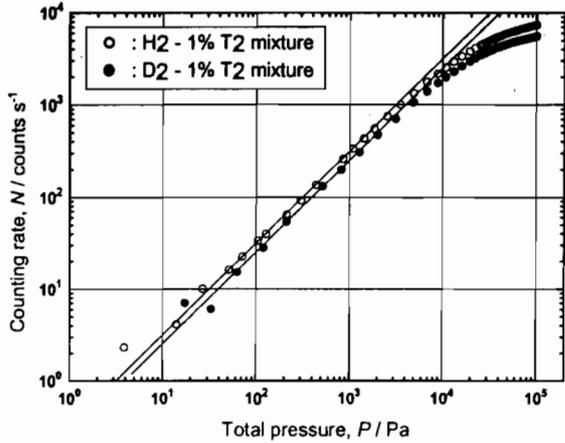
Fig. 3 Pressure dependence of X-ray intensity for the H<sub>2</sub>- and D<sub>2</sub>-1%T<sub>2</sub> mixtures.
