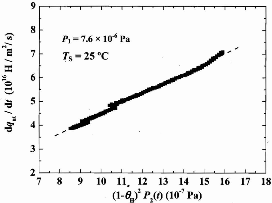
Fig. 8 Correlation between the rate of hydrogen uptake,  $q_{ut} / dt$ , and  $(1-\theta_H)^2 \cdot P_2(t)$  at 25 °C.
