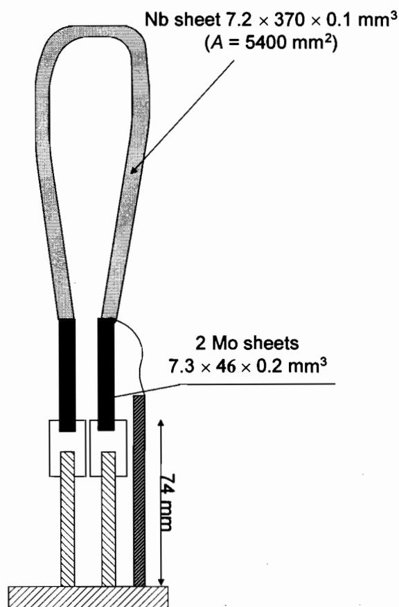
Fig. 1 Schematic description of specimen setup.
