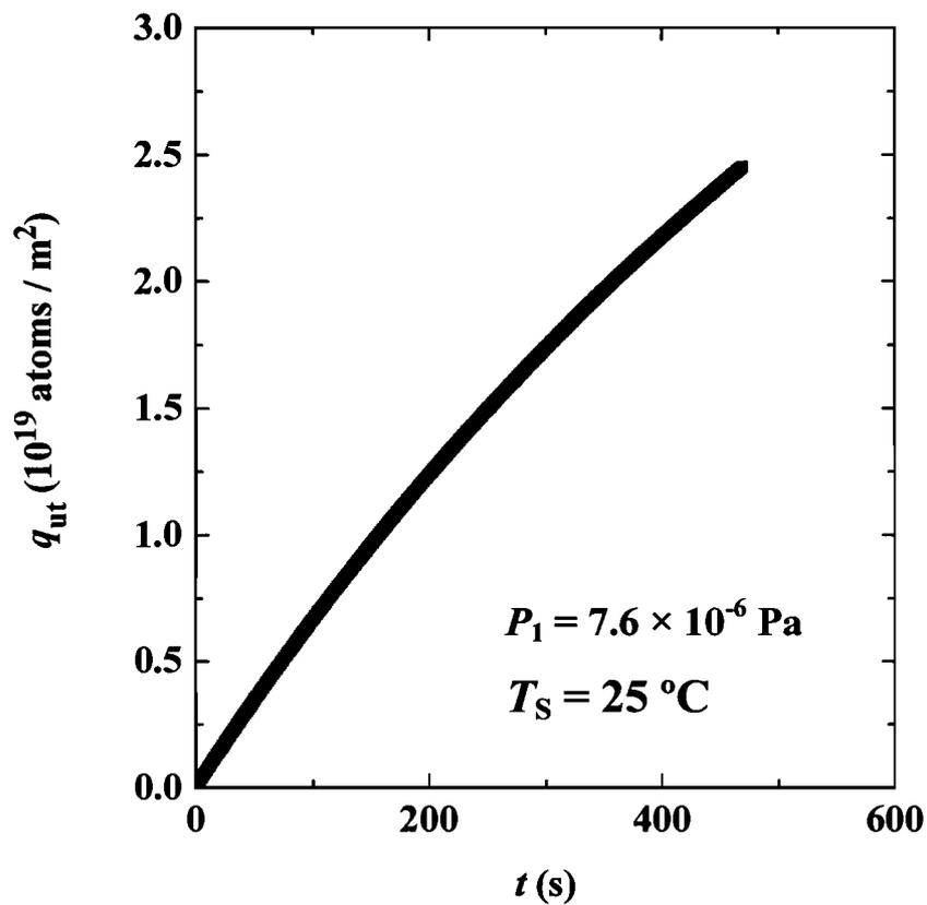
Fig. 6 Change in hydrogen uptake  $q_{ut}$  with time  $t$  at  $25\text{ }^\circ\text{C}$ .
