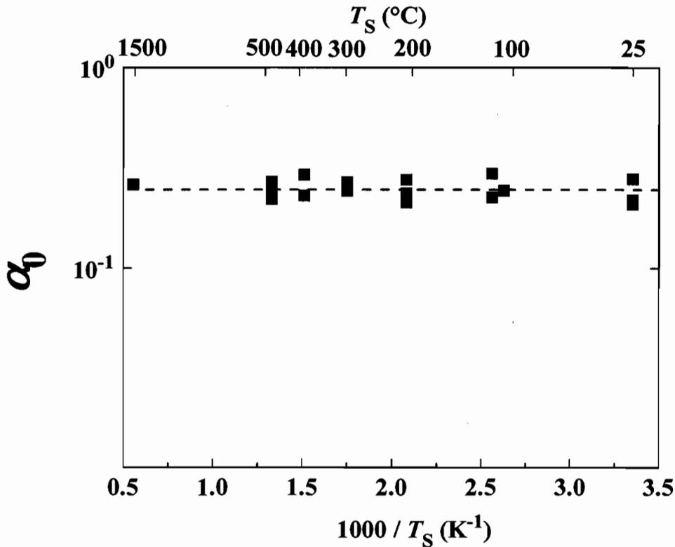
Fig. 5 Temperature dependence of initial sticking coefficient,  $\alpha_0$ .
