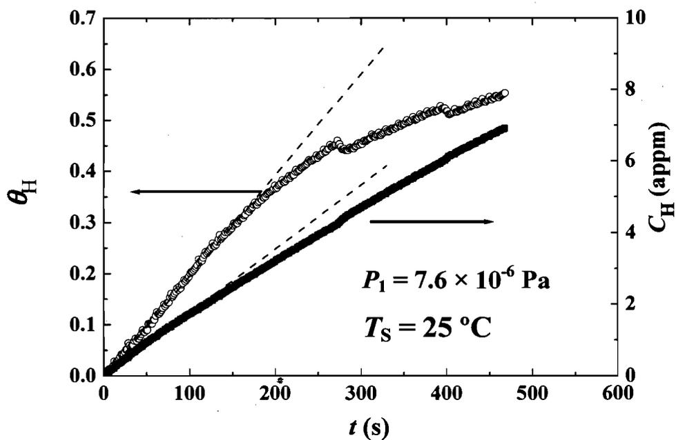
Fig. 7 Changes in  $\theta_H$  and  $C_H$  with  $t$  at  $25\text{ }^\circ\text{C}$ .
