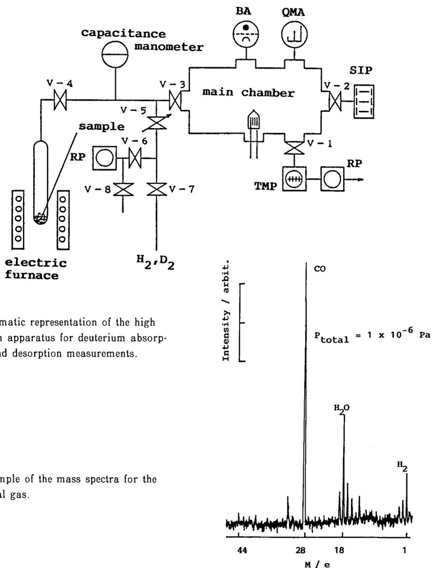
Fig.1. Schematic representation of the high vacuum apparatus for deuterium absorption and desorption measurements.
