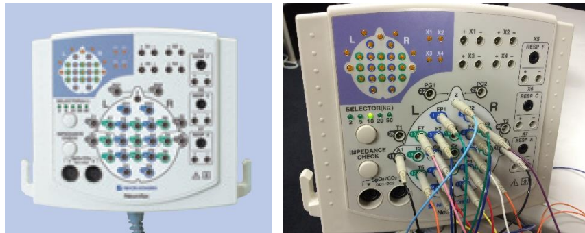
Figure 9. Electrode junction box
