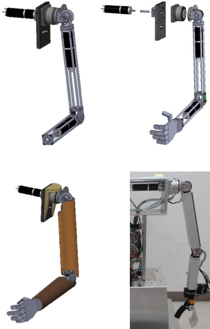
**Figure 3-4** Left hand design of the mobile humanoid robot.
