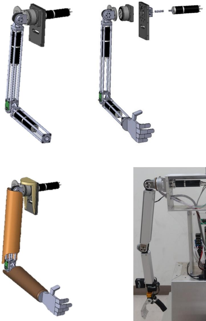
**Figure 3-3** Right hand design of the mobile humanoid robot.
