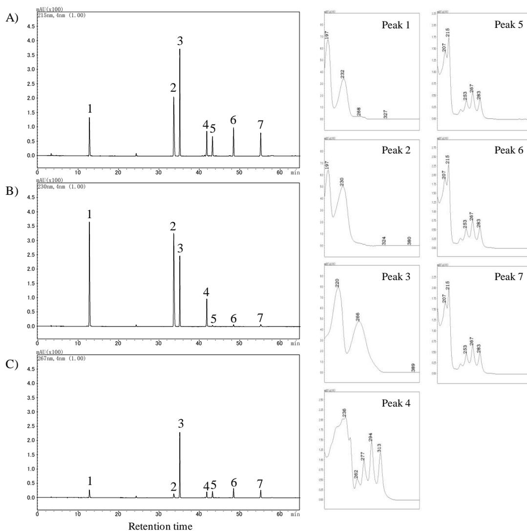
Fig. 2.4 HPLC chromatograms of a mixture of seven standard compounds (left panel) and UV spectrum of the respective compounds (right panel)
