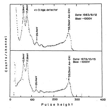
Fig. 6 Comparison of  $\gamma$ -ray spectra obtained from HgI<sub>2</sub> detector (1×1.6×0.5mm<sup>3</sup>), (upper) on Aug. 12, 1983 and (lower) on Oct. 15, 1978
