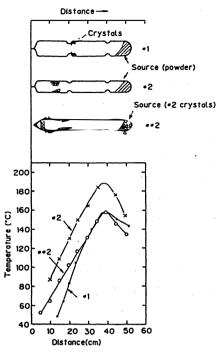
Fig. 1 Positions of crystals grown and corresponding temperature distributions
