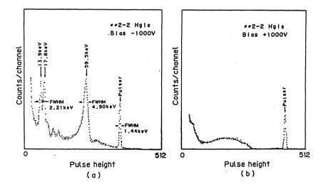
Fig. 4  $^{241}\text{Am}\ \gamma\text{-ray}$  spectra obtained from HgI<sub>2</sub> detector (1. 95mm<sup>2</sup>  $\times$  0.7mm) with (a) -1,000 V bias and (b) +1,000 V bias at room temperature
