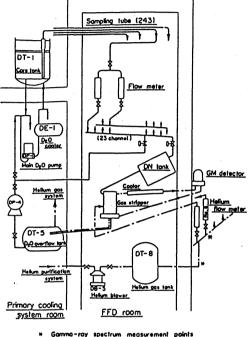
Fig. 7  $\gamma$ -ray spectrum measurement
