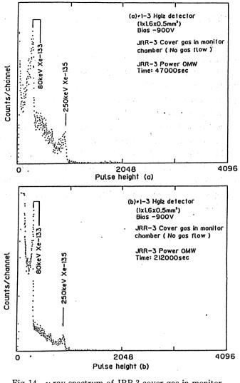
Fig. 14  $\gamma$ -ray spectrum of JRR-3 cover-gas in monitor chamber obtained from HgI<sub>2</sub> detector after covergas flow was shut off
