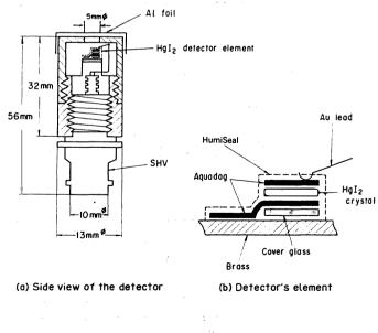
Fig. 2 Structure of detector and its element
