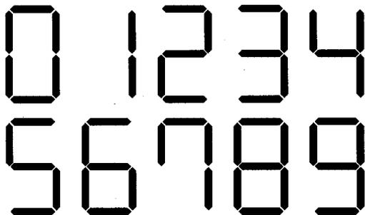
Fig. 3 Number patterns displayed on a seven-segment display.
