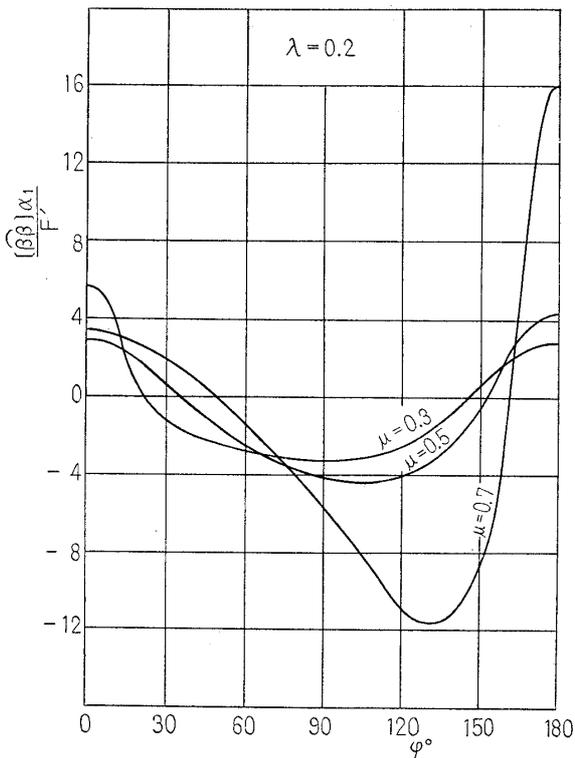
Fig. 3 Stress curves along hole when  $\lambda=0.2$ , where  $F'=F/(1/4\pi R_2)$
