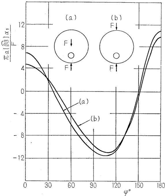
Fig. 2 Stress curves along hole, under radial or diametral forces, when  $\lambda=0.176$  and  $\mu=0.525$
