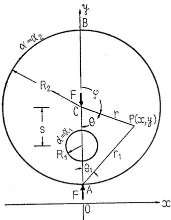
Fig. 1 Disk with an eccentric hole loaded at its centre and periphery
