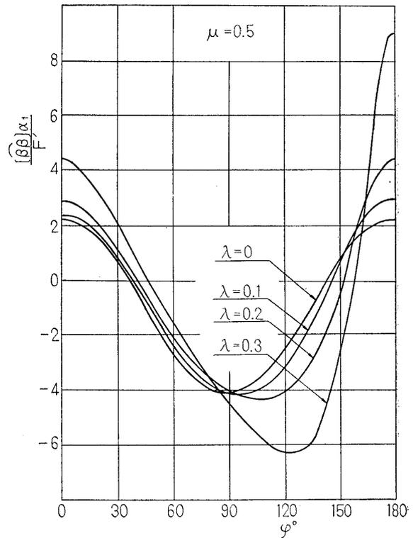
Fig. 4 Stress curves along hole when  $\mu=0.5$  where  $F'=F/(1/4\pi R_2)$
