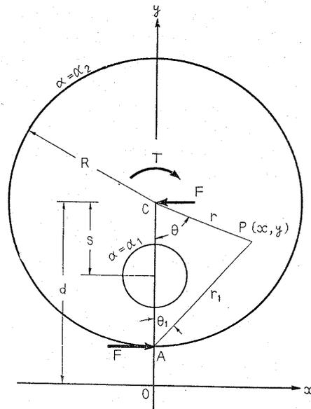
Fig. 1 Disk with an eccentric hole loaded at its center and periphery
