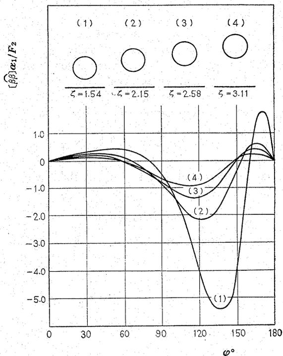
Fig. 5 Stress curves along hole in semi-infinite plate
