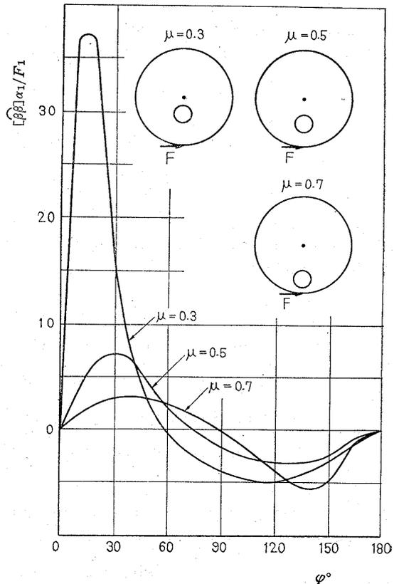
Fig. 3 Stress curves along hole when  $\lambda = 0.2$ , where  $F_1 = 4F/\pi a \operatorname{cosech} \alpha_2$
