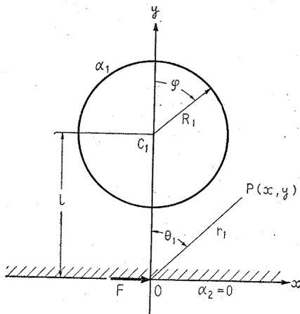
Fig. 2 Semi-infinite plate with a hole loaded at its straight edge
