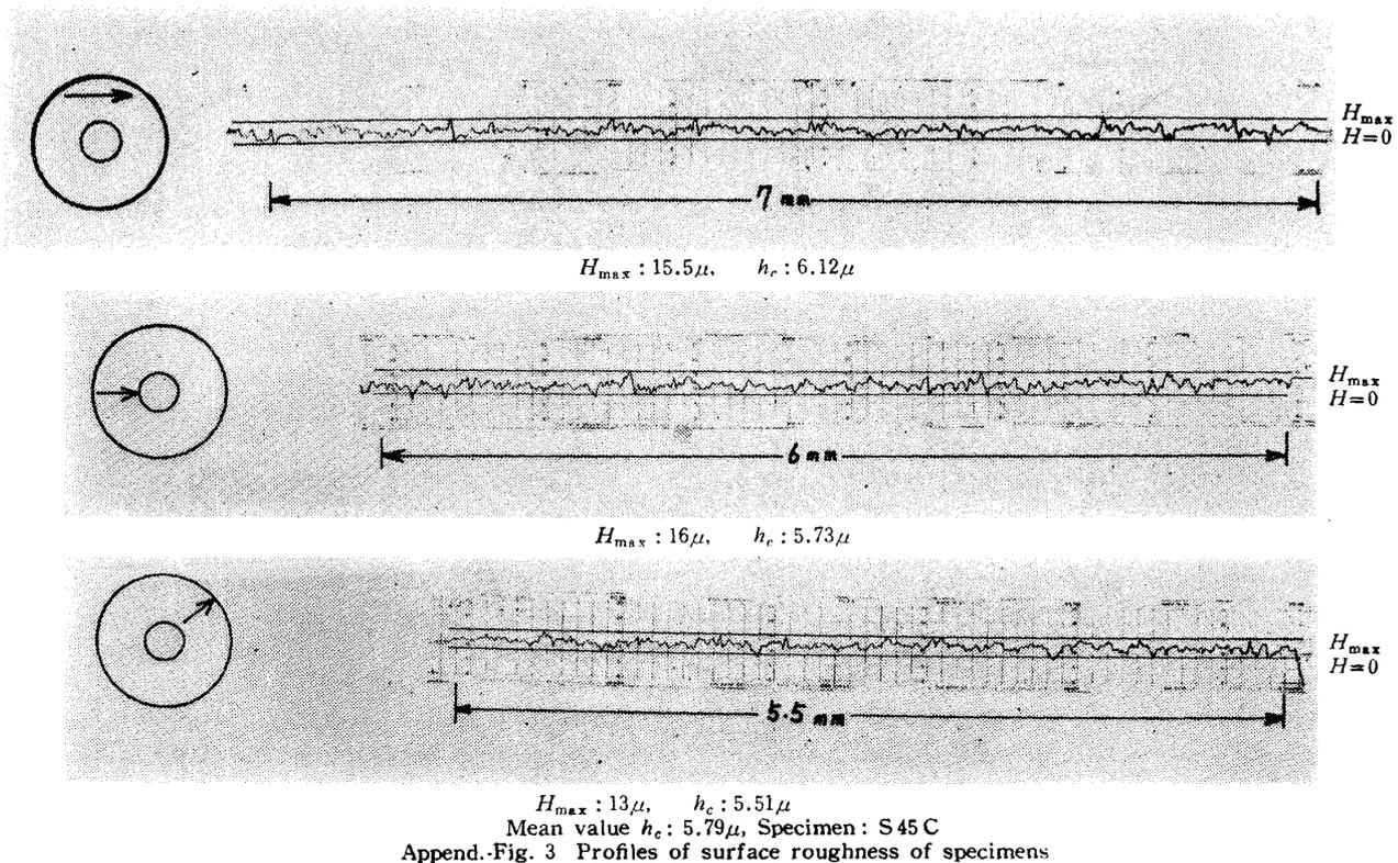
Append.-Fig. 3 Profiles of surface roughness of specimens
