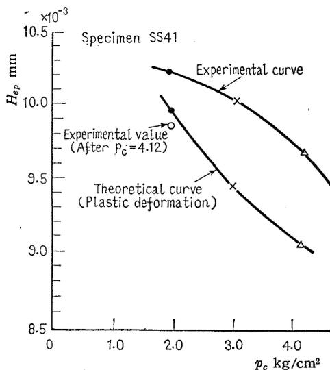
Fig. 19 Characteristic curves ; applied load versus equivalent gap
