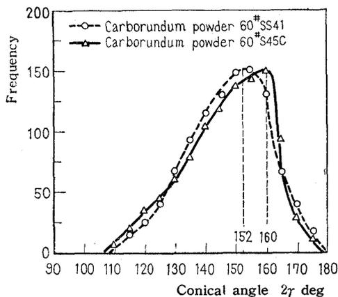
Fig. 10 Distribution of conical angle of surface irregularities
