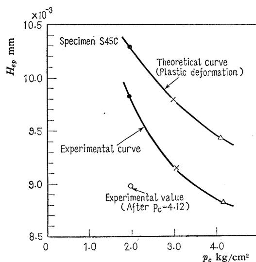
Fig. 20 Characteristic curves ; applied load versus equivalent gap
