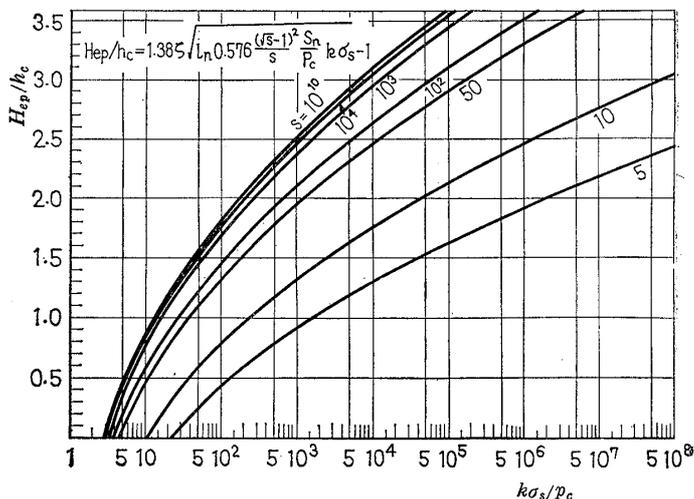
Fig. 4 Characteristic curves; assumed that the truncated cones are ideally plastic
