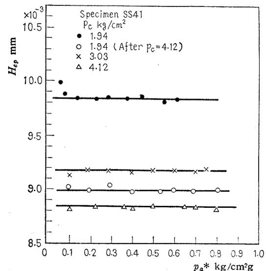
Fig. 18 Values of equivalent gap of experimental results
