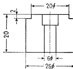
Fig. 8 Form of specimens
