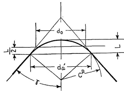
Fig. 13 Calculation method of dimension  $d_0$
