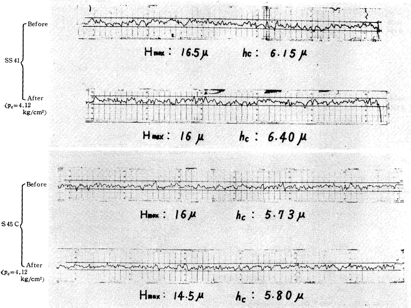
Append.-Fig. 7 Comparison of profiles of surface roughness
