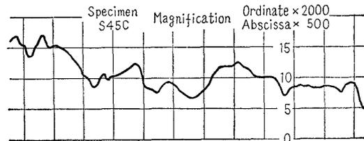
Fig. 12 Enlarged profile of surface irregularities
