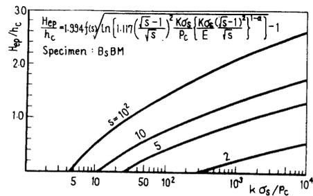
Fig. 14 Characteristic curves: assumed that the deformation of truncated cone is elasto-plastic
