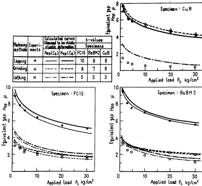
Fig. 7 Relation between applied load and equivalent gap
