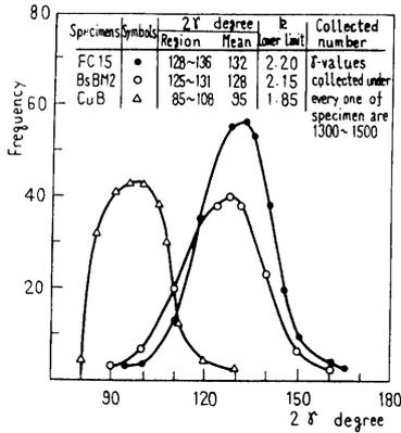
Fig. 3 Distribution of conical angles of surface irregularities (Finishing: Lapping)
