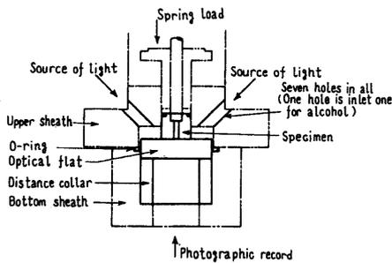
Fig. 8 Procedure of observation of leakage flow between contact surfaces
