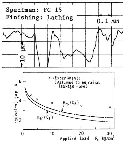
Fig.11 Comparison of the experimental and the calculated values of equivalent gap, where cavity exists in some region of the contact surface of specimen and the surface roughness is rough
