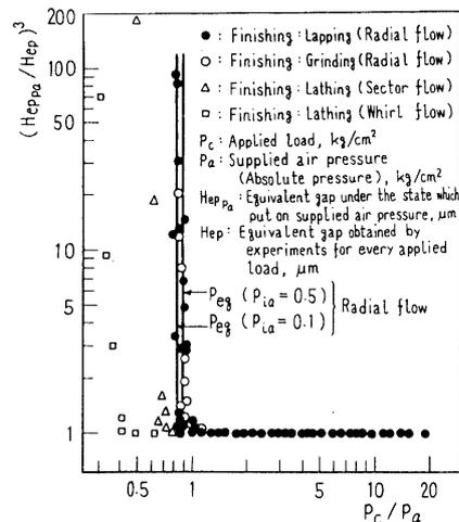
Note: Leakage flow between contact surfaces is assumed to be radial one
