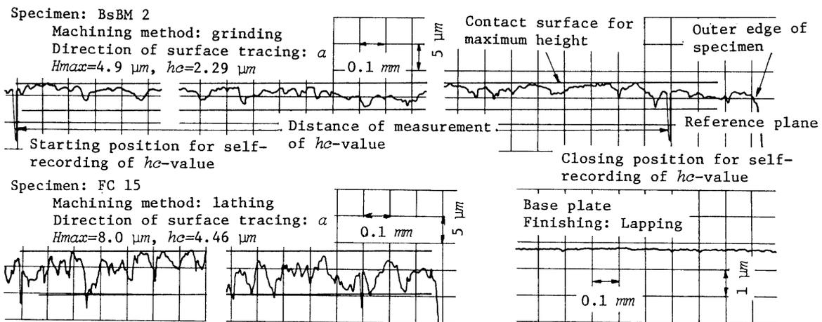
Fig. 1 Profiles of surface roughness of specimen and base plate (before the measurement)
