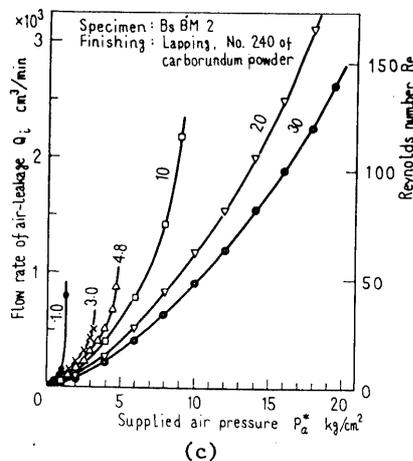
Note: Numerical values for every curve are applied load indicated in  $\text{kg/cm}^2$
