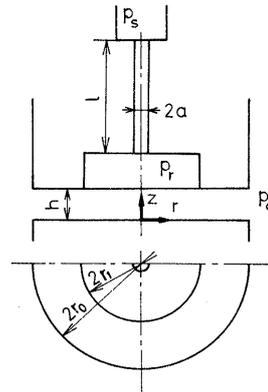
Fig.1 Coordinate system for thrust bearing
