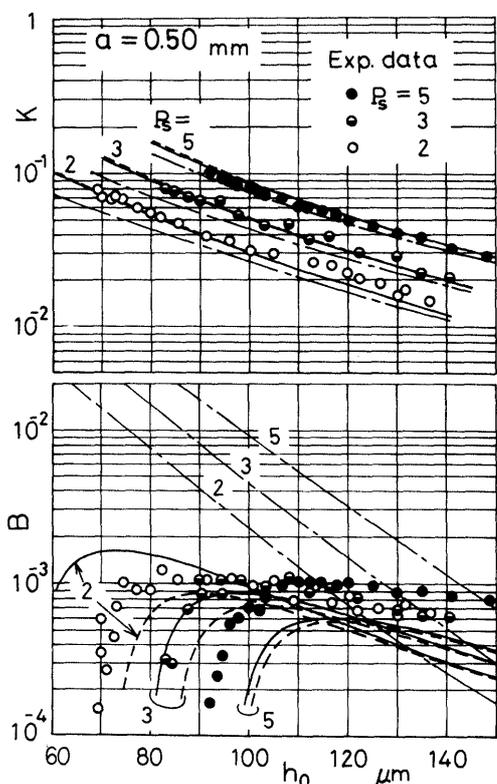
Fig.8 Comparison with experiment ( Bearing 1 )
