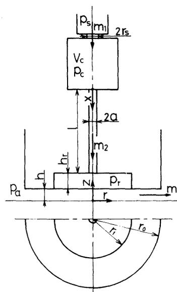
Fig.1 Coordinate system for thrust bearing
