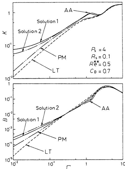
Fig. 3 Comparison of approximate solutions for dynamic stiffness and damping coefficient
