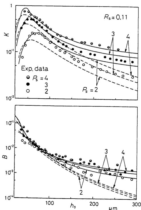
Fig. 6 Results of Solution 1 and the classical lubrication theory compared with experiment, for dynamic stiffness and damping coefficient
