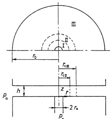
Fig. 1 Schematic diagram of externally pressurized thrust bearing
