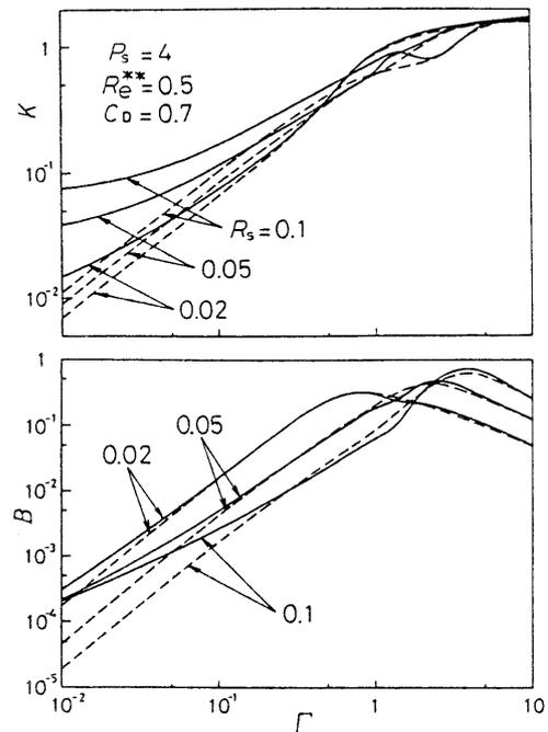
Fig. 4 Dynamic stiffness and damping coefficient for different radii of supply hole  $R_s$
