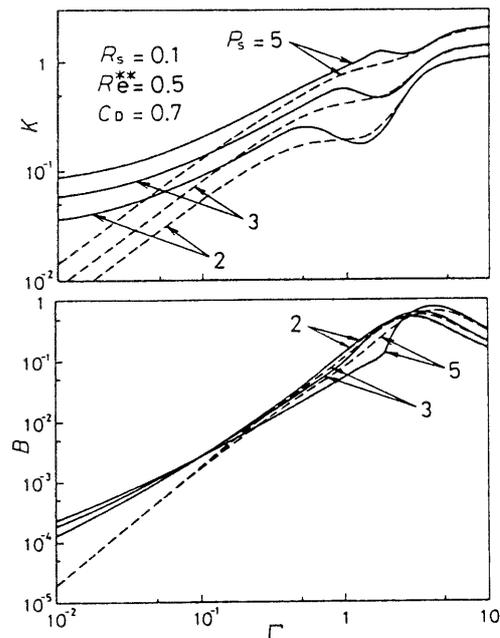
Fig. 5 Dynamic stiffness and damping coefficient for different supply pressures  $P_s$
