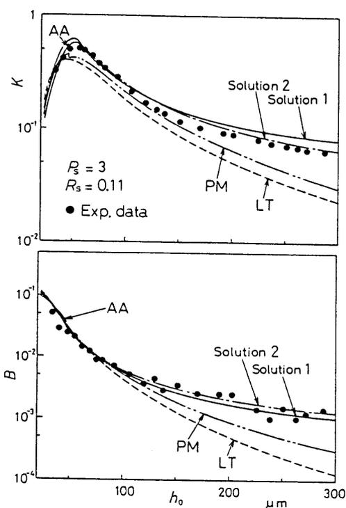
Fig. 7 Results of various analytical models compared with experiment, for dynamic stiffness and damping coefficient
