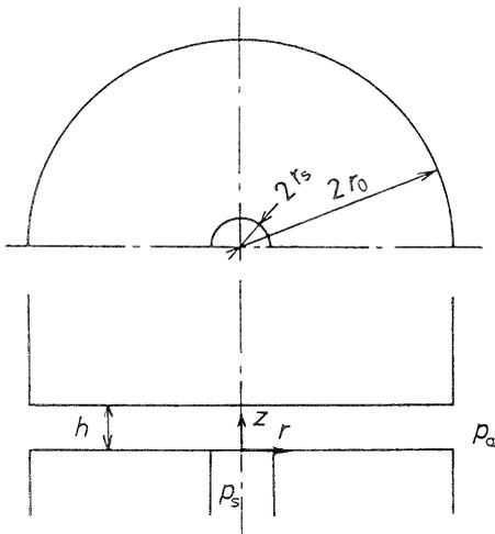
Fig. 1 Schematic view of externally pressurized thrust bearing with a single central supply hole
