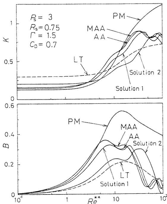
Fig. 2 Comparison of approximate solutions for dynamic stiffness and damping coefficient
