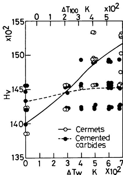
Fig. 4 Variations of micro-Vickers hardness through thermal shock
