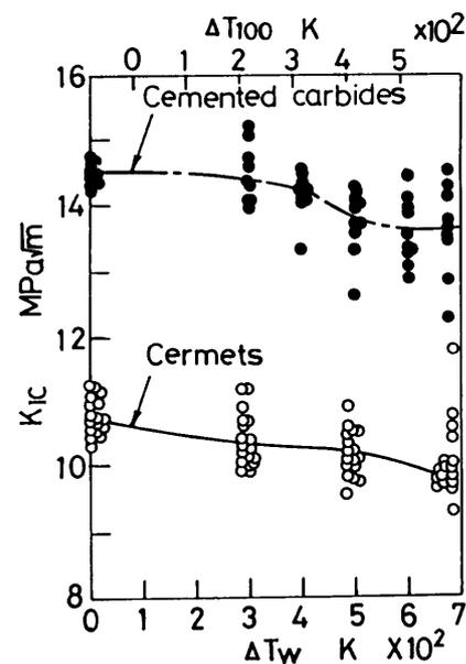
Fig. 5 Variations of fracture toughness through thermal shock
