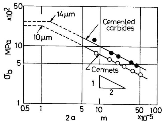
Fig. 8 Relationship between bending strength  $\sigma_b$  for the precracked specimens and precrack length  $2a$
