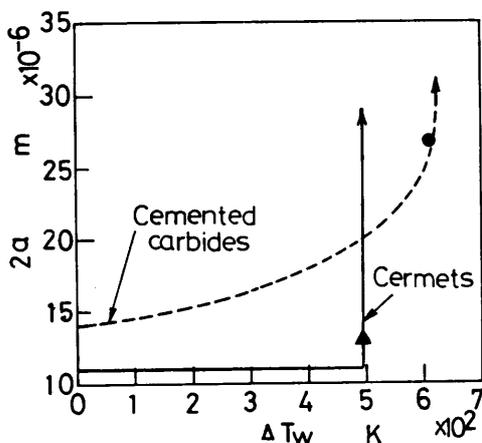
Fig. 9 Estimated crack growth curves during the thermal shock tests
