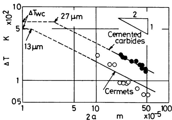
Fig. 7 Relationship between crack length  $2a$  and  $\Delta T$  at which the precrack starts to grow to about  $10 \mu\text{m}$
