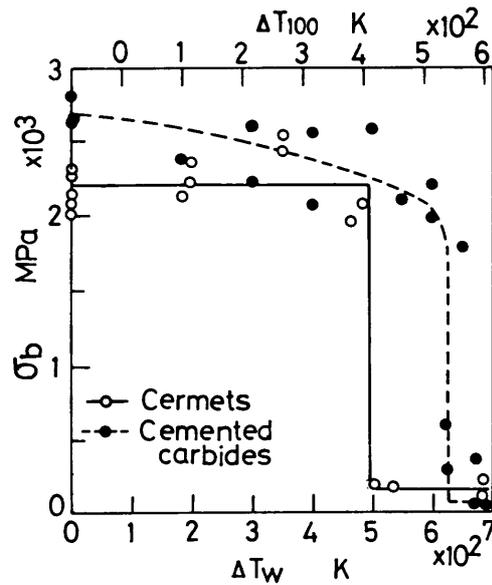
Fig. 3 Variations of bending strength due to thermal shock
