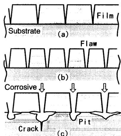
Fig. 11 Schematic illustration to explain the formation of corrosion pits and crack initiation of specimen with preflawed TiN coating film
