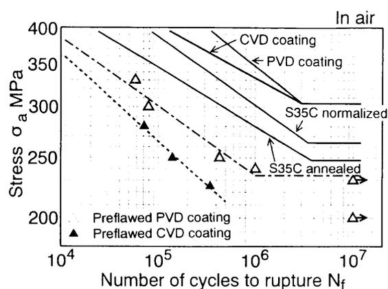
Fig. 3 S-N diagram for fatigue test in air using specimens with preflawed coating film
