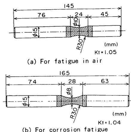
Fig. 1 Shape and dimensions of fatigue test specimens; (a) for fatigue tests in air, and (b) for corrosion fatigue tests in saline solution
