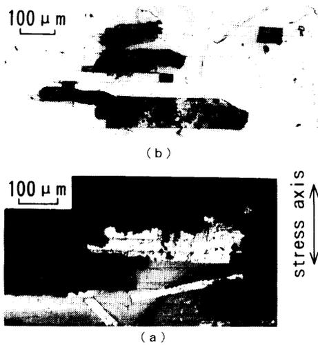
Fig. 7 Surface morphology of specimen with preflawed PVD coating film after corrosion fatigue testing: (a) preflaw density  $\rho = 47/\text{mm}$ ,  $\sigma_a = 150 \text{ MPa}$ , and (b)  $\rho = 24/\text{mm}$ ,  $\sigma_a = 250 \text{ MPa}$
