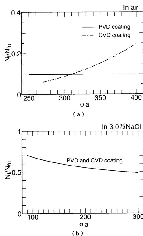
Fig. 5 Decrease in fatigue life of specimens with preflawed coating film: (a) fatigue in air, and (b) corrosion fatigue in saline solution
