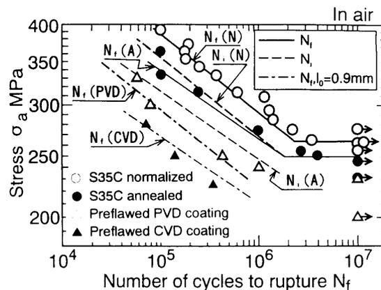
Fig. 13 Estimation results of fatigue life in air for specimen with preflawed coating film
