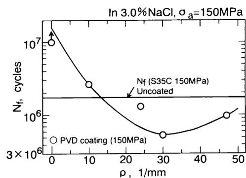
Fig. 6 Relationship between corrosion fatigue life in PVD coated specimen and preflaw density in coating film determined from experiment ( $\sigma_a=150$  MPa)
