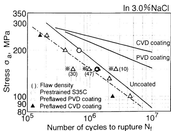
Fig. 4 S-N diagram for corrosion fatigue test in 3.0% NaCl saline solution using specimens with preflawed coating film
