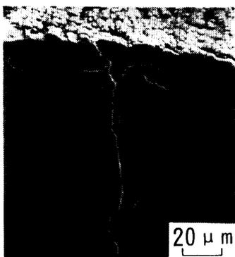
Fig. 12 SEM observation of the cross section of a CVD-coated specimen showing corrosion pits and a crack just below flaws in the coating film
