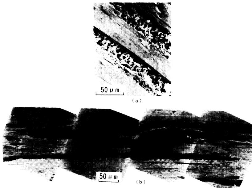
Fig. 8 SEM observation of surface of specimen with preflawed PVD coating film under corrosion fatigue testing
