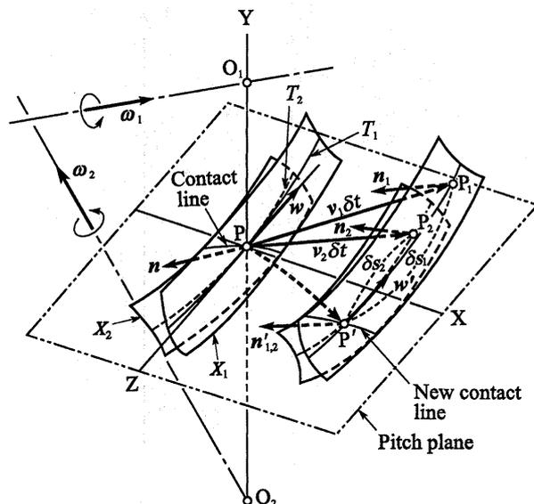
Fig. 3 Tooth surface mesh with a contact line
