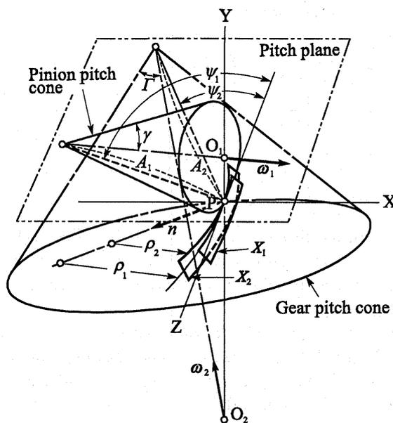
Fig. 5 Pitch cones of hypoid gears on their pitch plane
