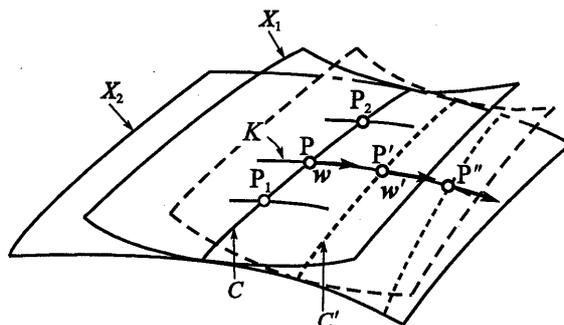
Fig. 1 Relative motion of two surfaces and a slide line
