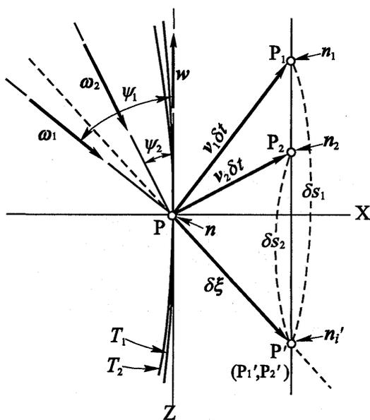
Fig. 4 Tooth spiral after small incremental relative motion
