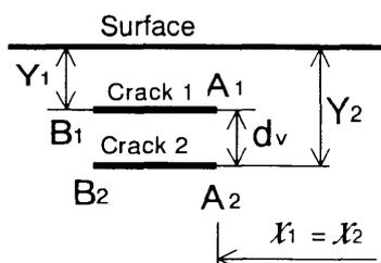
Fig. 3 Two subsurface cracks arranged in a row
