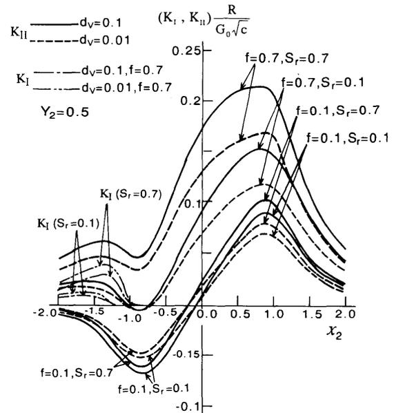
Fig. 9 Stress intensity factors  $K_{II}$  as a function of crack location for the case of  $Y_2=0.5$
