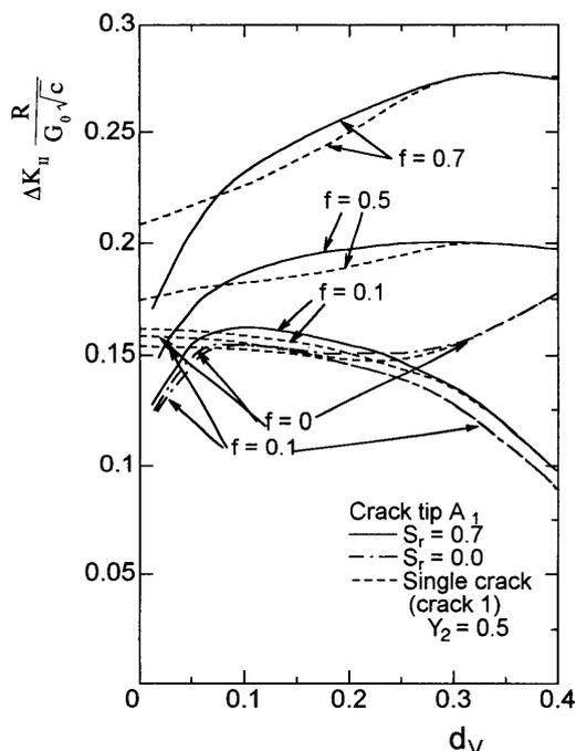
Fig. 11 Interference effects on  $\Delta K_{II}$  of the crack tip  $A_1$  with a decrease of  $d_v$  for  $Y_2=0.5$ ,  $S_r=0$  and  $0.7$
