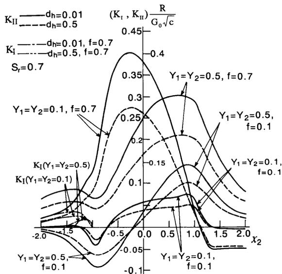
Fig. 5 Stress intensity factors  $K_{II}$  as a function of crack location for the case of  $S_r=0.7$
