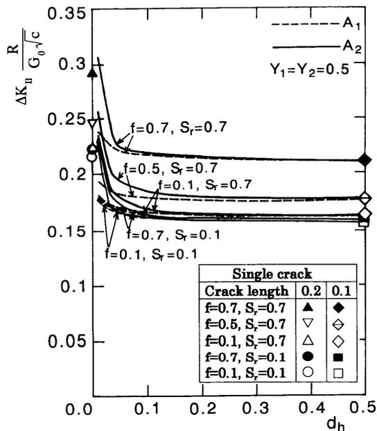
Fig. 7 Interference effects on  $\Delta K_{II}$  with a decrease of  $d_h$  for the case of  $Y_k=0.5$ ,  $S_r=0.1$  and  $0.7$
