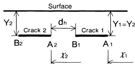
Fig. 2 Two subsurface cracks arranged in a series
