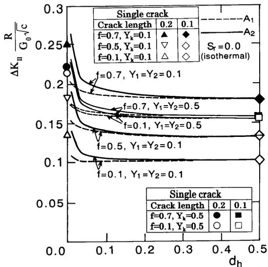
Fig. 6 Interference effects on  $\Delta K_{II}$  with a decrease of  $d_h$  for isothermal case ( $S_r=0$ )
