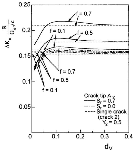
Fig. 10 Interference effects on  $\Delta K_{II}$  of the crack tip  $A_2$  with a decrease of  $d_v$  for  $Y_2=0.5$ ,  $S_r=0$  and  $0.7$
