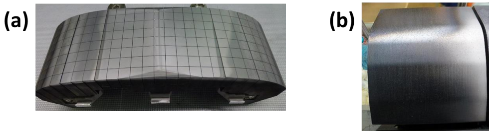
Fig. 1.11. Photo of JET-ILW (a) Be limiter tile IWGL and (b) W-CFC divertor Tile 1.
