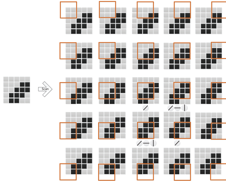
Figure 2.4: Diagram of the judgment of global planar orientation detection by the local planar orientation-detective neurons.
