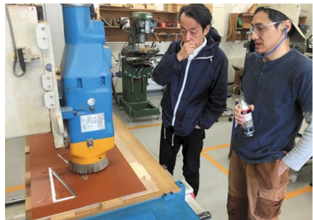
Photo 8: cutting out Duralumin beam at the faculty's workshop
