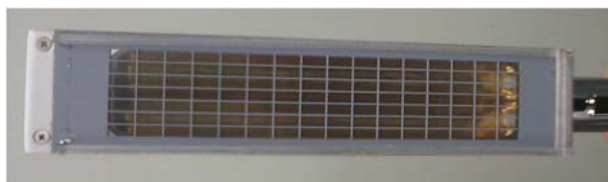
Fig. 9 Photo of a \beta -ray detector for tritium measurement. Thin membrane of the entrance window is 0.15 \text{ mg/cm}^2 in thickness.
