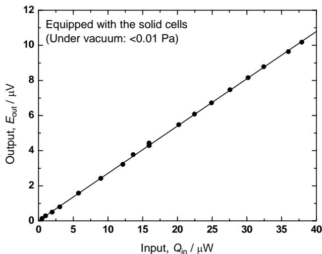
Fig. 11 Calibration curve for the solid tritium measurements.
