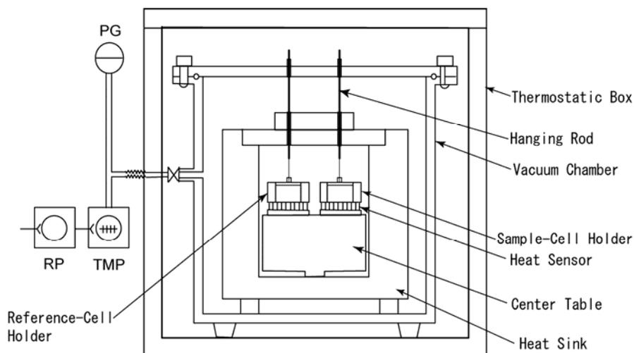
Fig. 4 Schematic drawing of a specially designed high sensitivity calorimeter.
