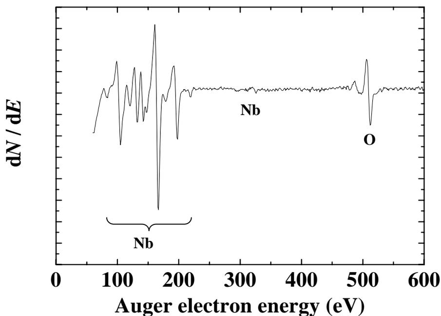
Fig. 3 Typical example of Auger spectra obtained at 1113 K for the specimen containing 1 at% of oxygen.
