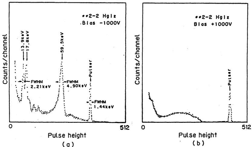
Fig. 4  $^{241}\text{Am}$   $\gamma$ -ray spectra obtained from  $\text{HgI}_2$  detector ( $1.95\text{mm}^2 \times 0.7\text{mm}$ ) with (a)  $-1,000\text{V}$  bias and (b)  $+1,000\text{V}$  bias at room temperature
