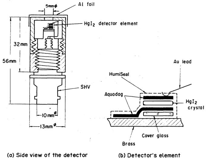
Fig.2 Structure of detector and its element
