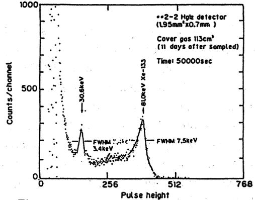
Fig.9  $\gamma$ -ray pulse height distribution obtained from HgI<sub>2</sub> detector (1.95mm $\times$ 0.7mm) with -1,000 V bias at room temperature
