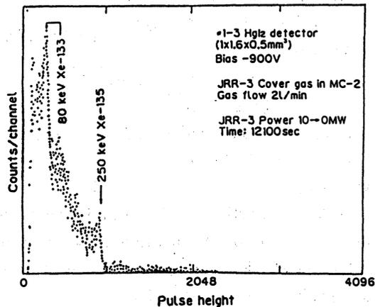
Fig. 13 JRR-3 cover-gas  $\gamma$ -ray spectrum obtained from  $\text{HgI}_2$  detector with -900 V bias at room temperature
