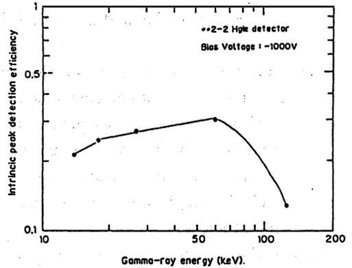
Fig. 11 Intrinsic peak detection efficiency of #2-2  $\text{HgI}_2$  detector
