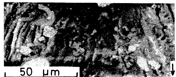
(a) \sigma=220 MPa, \Delta K=2\text{MPa}\cdot\text{m}^{1/2}
