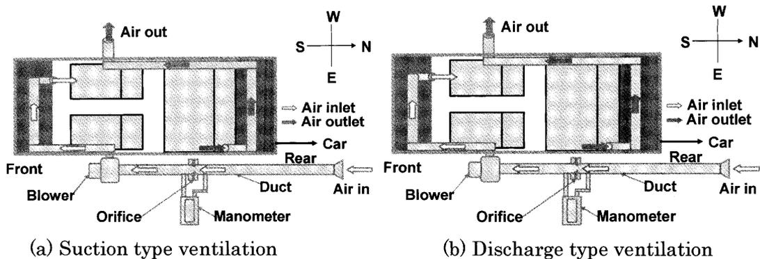
Fig. 2 Schematic diagram of experimental setup for flow rate measurement
