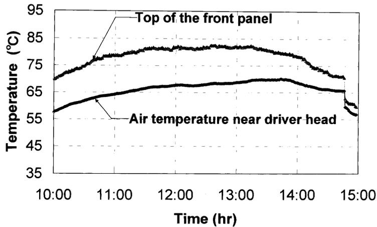
Fig. 3 Temperature variation with time at different locations (without cooling)
