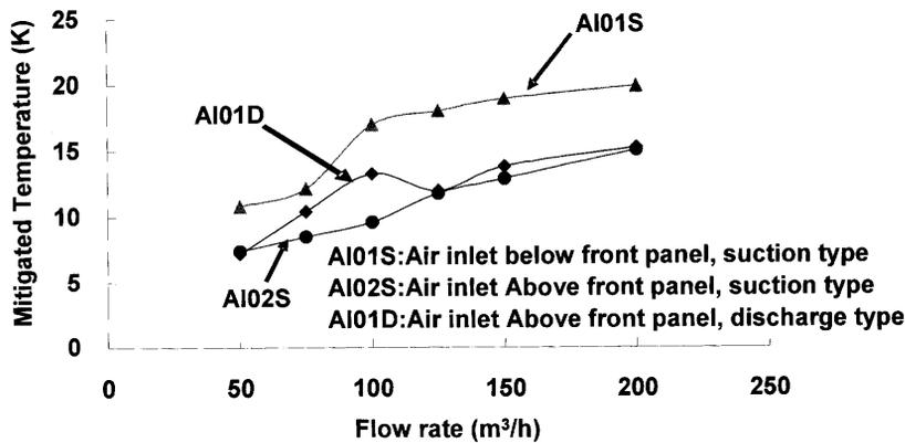
Fig.5 Effect of different air inlet locations and different ventilation methods on temperature mitigation
