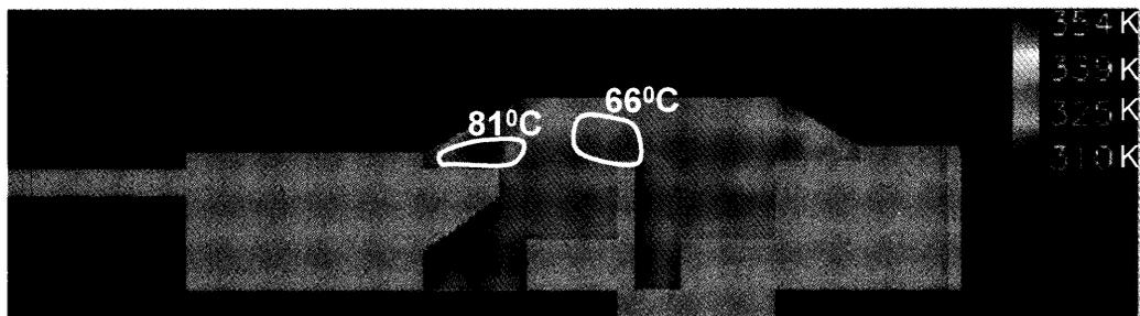
Fig. 7 Temperature distribution in the car cabin without ventilation (Section X-Y)
