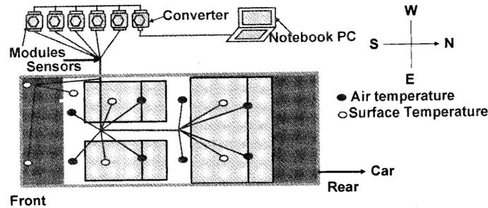
Fig. 1 Schematic diagram of experimental setup for temperature measurement
