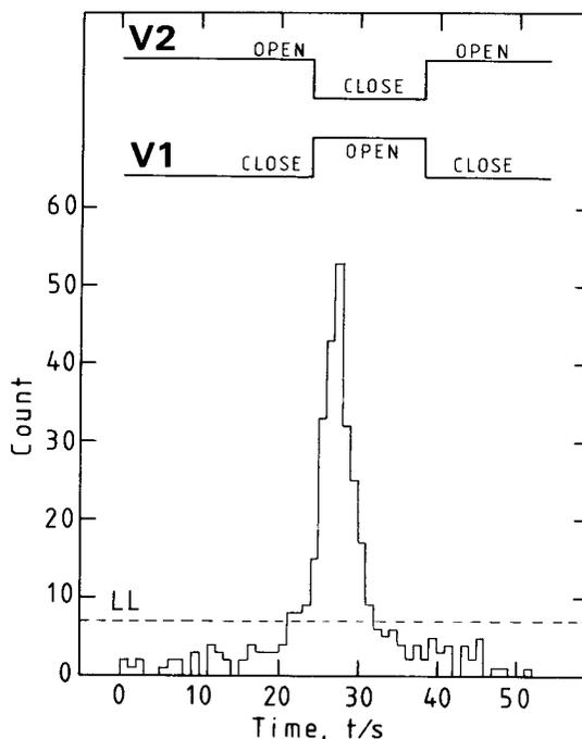
Fig. 5 An example of the valve actions caused by artificial tritium flow.
