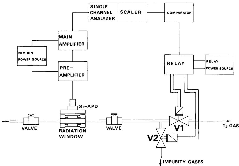
Fig.7 A schematic diagram of a changeover system of tritium flow channel.
