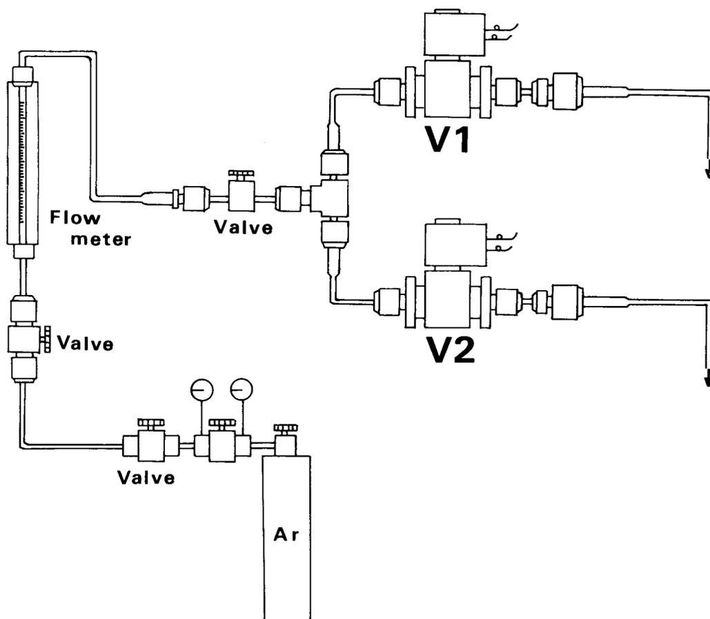
Fig.2 A schematic illustration of the valve connection in flow system.
