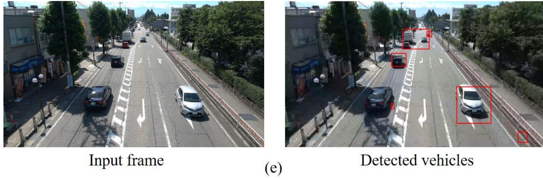
Figure 3.7: Detection results in uncompressed and compressed domain; (a) original video (92362 kbs), (b) compressed (9236 kbs), (c) compressed (739 kbs), (d) compressed (554 kbs), (e) compressed (462 kbs).
